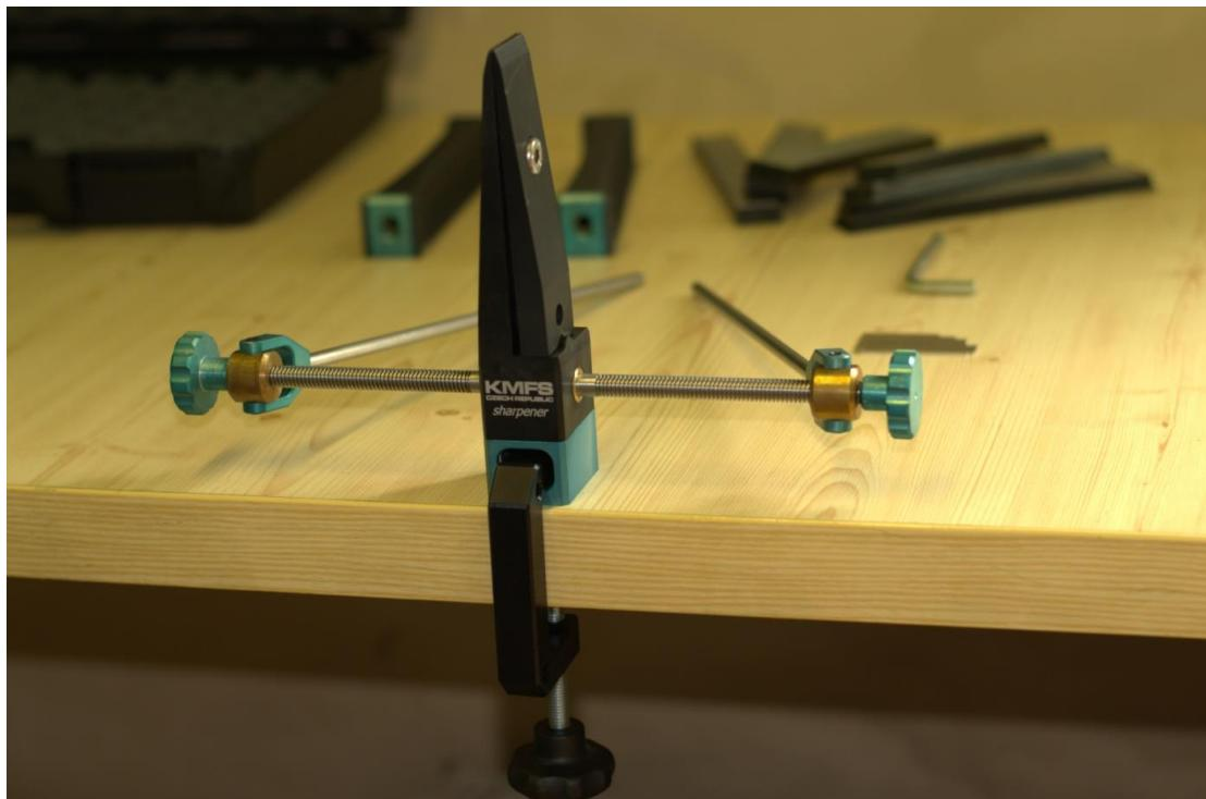
Insert the clamp in the clamp hole and use the plastic ring to fasten the clamp so that the knife vice is firmly fastened to the bench and cannot move.
