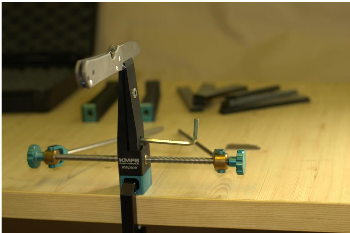
Now tighten the bottom knife vice screw counterclockwise so that the knife is fastened firmly and cannot move in the knife vice. The bottom knife vice screw is accessible through the hole on the right under the top knife vice screw.
