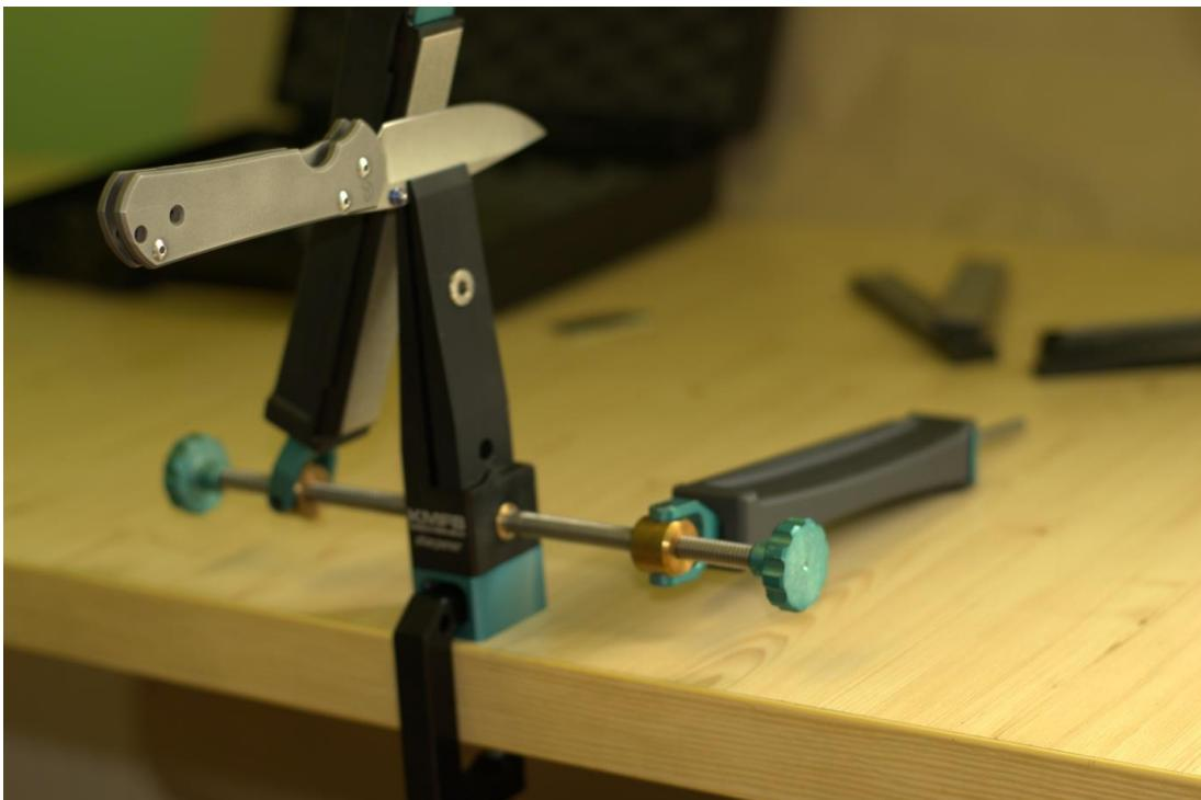
Now slide the left and right carriers alternately up and down the blade, so as to sharpen both sides of the knife identically. Do not stop sharpening using the coarsest whetstone until the sharpened surface extends all the way to the knife cutting edge. For better visibility, we recommend colouring the cutting edge with a black marker. The black line must not remain above the sharpened surface towards the cutting edge.
