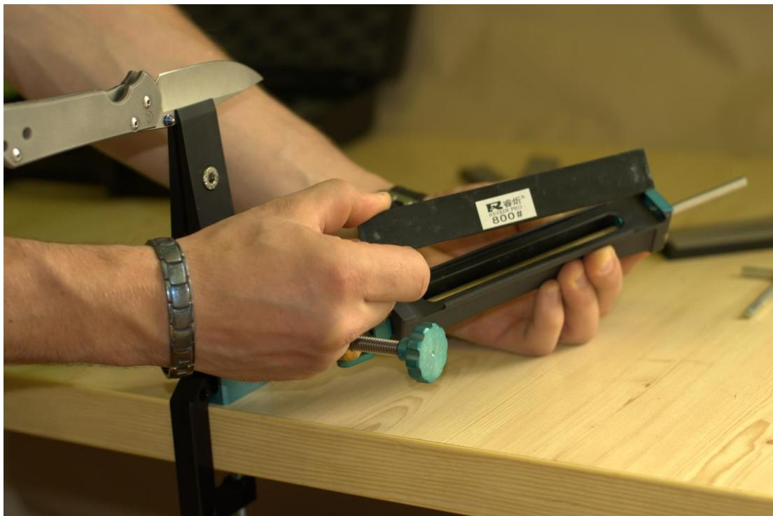
Now insert the whetstones with the highest number: the finest, and again sharpen until you completely erase all signs of previous sharpening.
