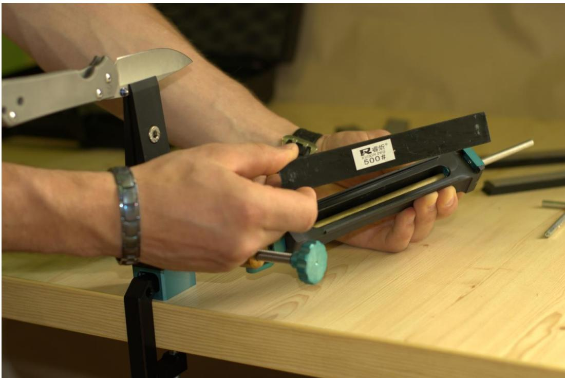
Replace the whetstone in both carriers with a finer one and again sharpen both sides of the blade until all signs of previous sharpening disappear.
