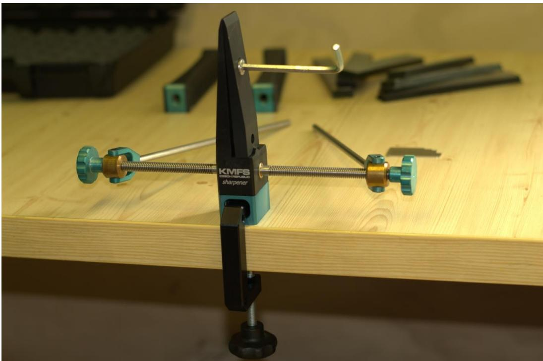
Use an Allen key to loosen the top screw of the knife vice so that the gap in the vice is wider than the thickness of the knife blade you are about to sharpen.
