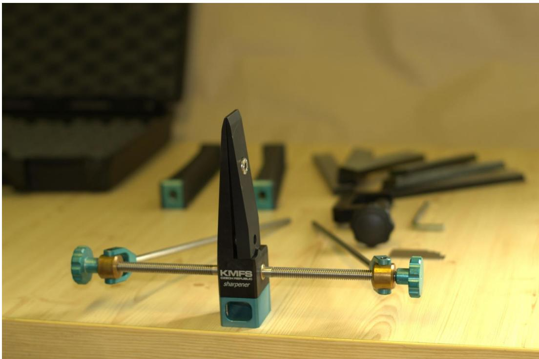
Place the kit on a firm workbench edge so that the hole for the clamp (in the blue cube at the bottom end of the knife vice) faces towards you.
